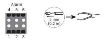
Figure 5.5 Alarm and relay connector pins
